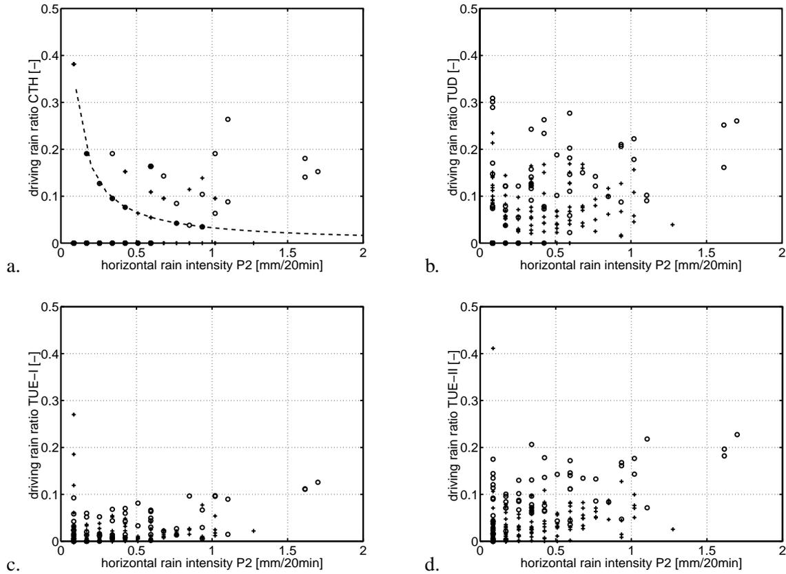
Figure 5: 20-min driving rain ratios  $R_f/R_h$  as function of horizontal rain intensity  $R_h$  and reference wind velocity component normal to the facade (+ = 4–5 m s<sup>-1</sup>, o = 6–7 m s<sup>-1</sup>).
