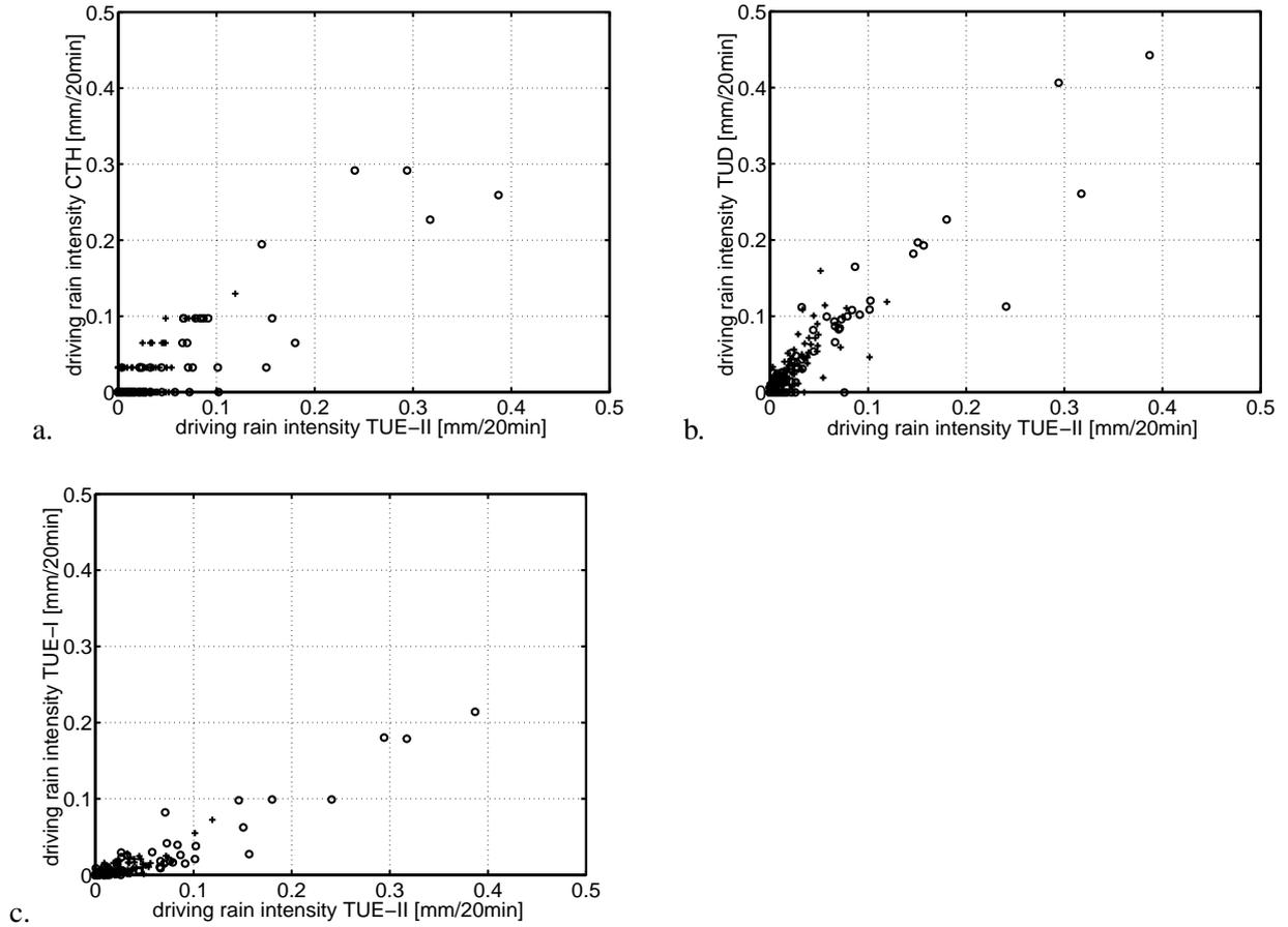
Figure 4: Correlation of 20-min driving rain intensities of gauge CTH, TUD and TUE-I with gauge TUE-II. Reference wind velocity normal to the facade: + = 4–5 m s<sup>-1</sup>, o = 6–7 m s<sup>-1</sup>.
