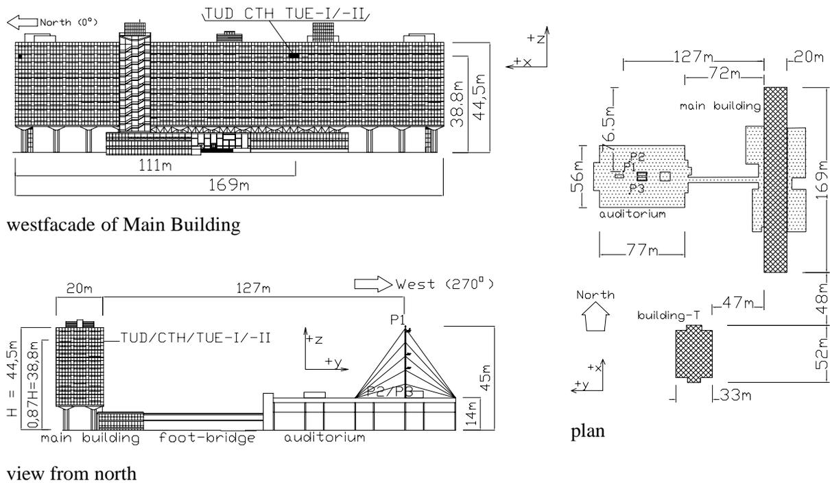
Figure 1: Test site, measurement positions and definition of  $x$ - $y$ - $z$  axis system.
