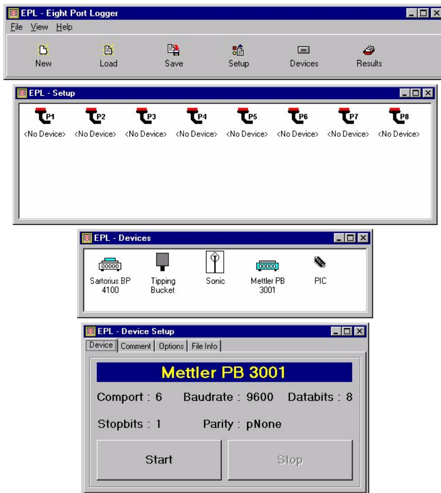
Figure 3.2: Eight Port Logger: the main, setup, devices and a device-setup window. Linking a device to a port is done by dragging the icon of a device in the devices window onto the icon of a port in the setup window. Then clicking onto a device in the setup window will give the device-setup window, by which the sample rate, device identification code etc, is defined. The command for starting or stopping the logging of the device is also done in this window. Results are shown in the results window (not shown here) and stored on disk.
